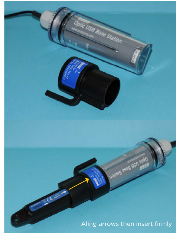
Optic base and coupler used for HOBOWARE HOBO-U22 data logger launching and offloading.
